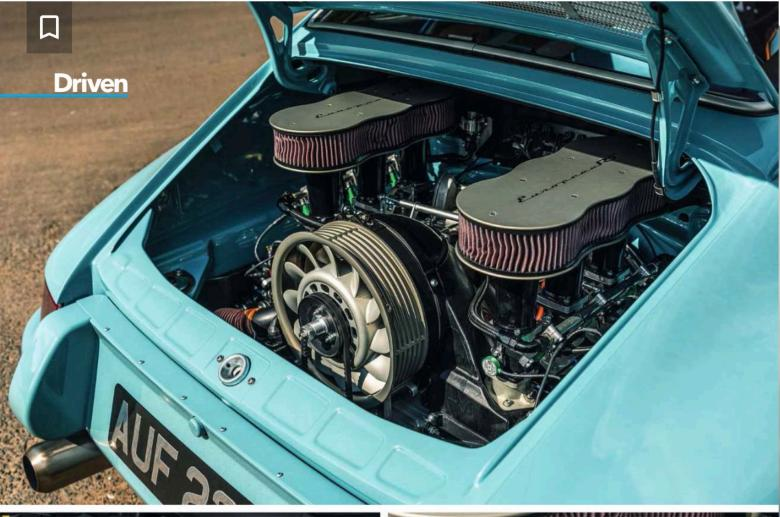
**Left:** engine is based on a 993 block, enlarged and significantly upgraded for 385bhp; red line is set at 8000rpm; other engine sizes and specs are offered
